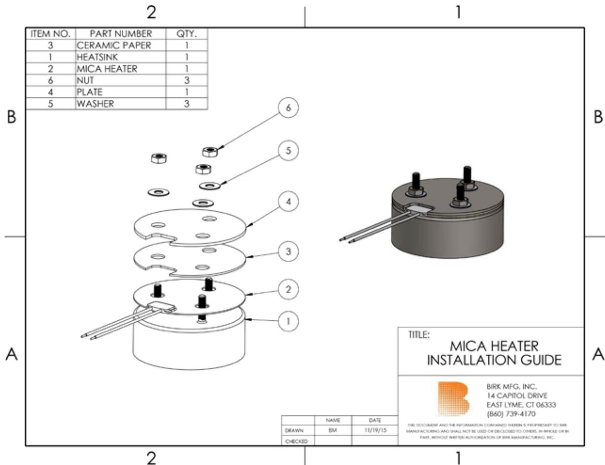
It is recommended that customers run their assembly at operating temperature for several hours before bringing back to a cooled state and ensuring all fasteners are securely tightened. Please note that during the initial temperature ramp-up the binder and insulating ceramic element provided with the heater will smoke slightly. This is normal and should not continue after the initial ramp-up.
